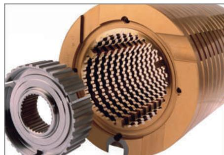
*Broaching process applied to outer circumferential shapes. Pot broaches are made up of special flat broaches and rings with internal profiles mounted inside cylindrical supports. This process is indicated for medium/high production of parts with complex external shapes.*
